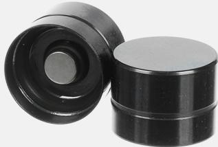
The working surface of the tappet is first perfectly polished and then the DLC layer is applied. The perfect polishing process is important so that the DLC layer blends perfectly with the base. The thickness of the DLC layer is 2-5 um. The achieved hardness is then more than 2000 HV.
