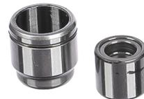
The bore in the tappet piston is made by double pressing, in order to achieve a suitable roundness that ensures even contact with the steel ball and optimal delivery of the amount of oil at the required time, thus extending the life of the part.
